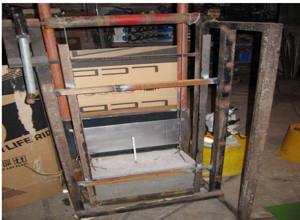
Figure 3: The radiation source and the bifilar pendulum with the sensor
